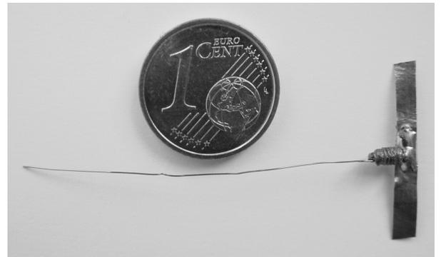
FIG 1. Reflector tag consisting of a silicium diode, a copper foil antenna and a copper wire antenna. The coin has a diameter of 16mm.
