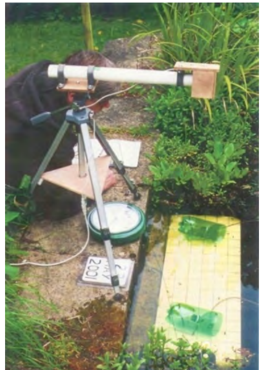
Figure 3. The video-recording set-up with a 30 x 80 cm laminate sheet defining the recorded area and the camera mounted over the area centre.
